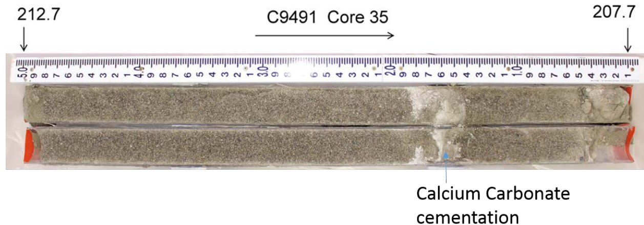
Figure 5: A small zone of calcium carbonate cementation is seen in borehole C9491. This is in a geographic area where carbonate cements are not typically observed at this depth.
